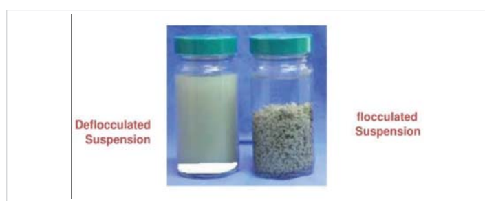
Figure 5: SUSPENSION deflocculated/flocculated. From Sahib.
