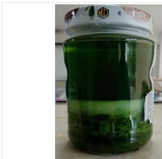
Figure 4: Extraction of Kalanchoe pinnata pulp using 99% acetone; the freshly prepared pulp of Kalanchoe pinnata leaves was extracted with 99% acetone in a 2:1 (v/w) ratio. The mixture was left for 72 hours before filtering to obtain the acetone extract.
